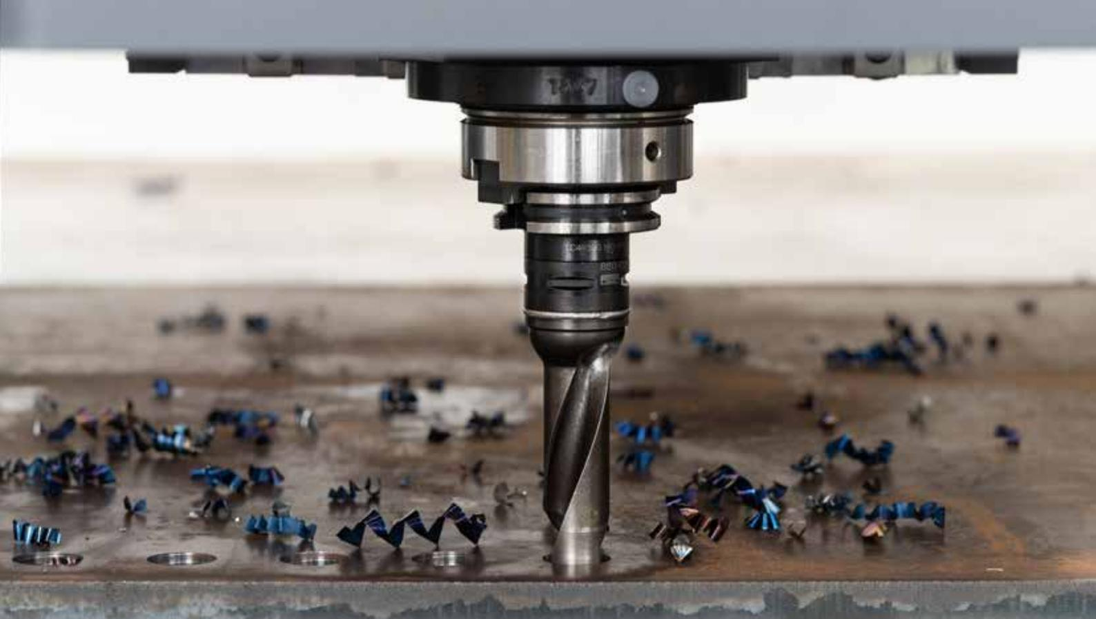
The newly designed hold-down clamp ensures stable support of the plate, thus ensuring low-vibration machining of the components. The integrated air nozzles efficiently remove chips and optimally prepare the system for subsequent processes.
